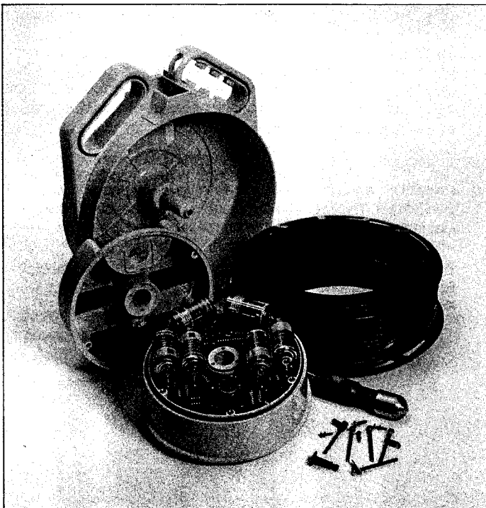
Electronics Housing, showing battery placement
